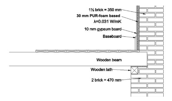
Figure 2. Section of internally insulated façade at Thomas Laubs Gade 5.
